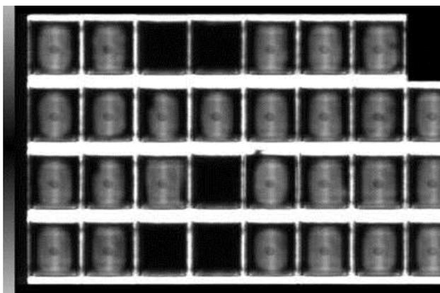
Fig. 10. CSAM images for 3<sup>rd</sup>lot: delamination in all parts
