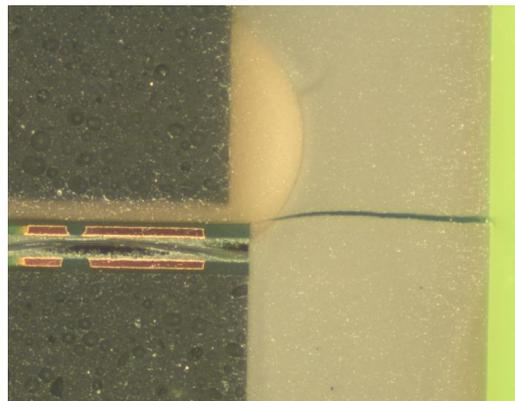
Fig. 8. X-section image of crack in the package
