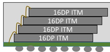
Fig. 2. 64DP Package-in-package construction
