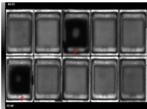
Fig. 7. CSAM image with delamination in 2 parts
