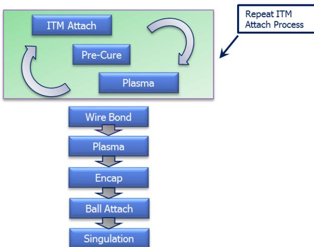
Fig. 3. Assembly process flow
