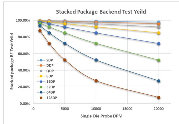
Fig. 1. Backend test yield vs. assumed probe DPM
