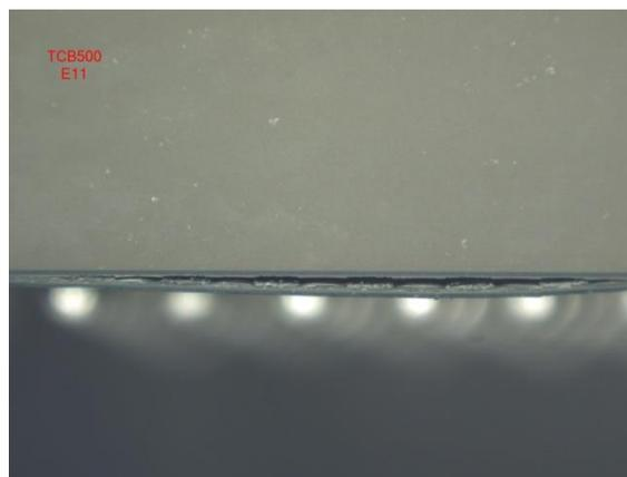
Fig. 9. Delamination between substrate and solder mask
