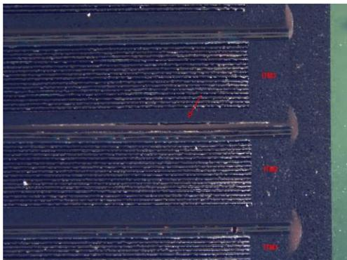
Fig. 11. X-section images of the delaminated part
