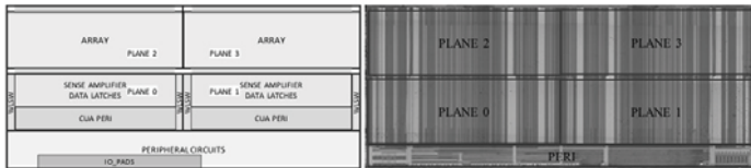
Figure 13.5.1: a) Key features (top). b) Chip Floorplan and Die photo (bottom).
