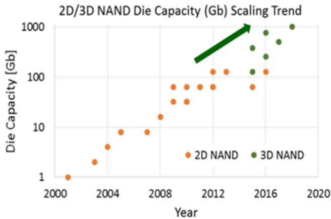
Fig. 1. Transition to 3D NAND has extended the die capacity scaling to 1Tb
