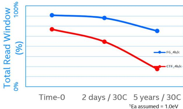
Fig. 7. Floating Gate Cell advantage for data retention
