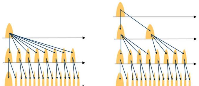
Fig. 4. 16 Level placement using 8-16 (64 layer) and 2-8-16 (96 layer) programming algorithm
