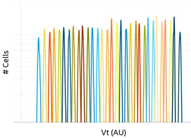
Fig. 8. Intel FG 3D NAND shows promise for 5 bits/cell
