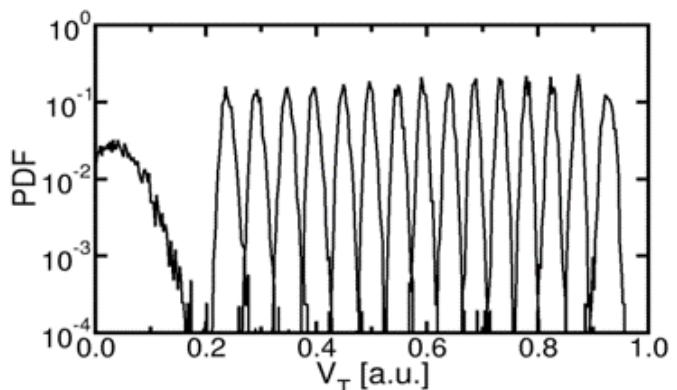
Fig. 6. V<sub>t</sub> distributions of cells in the 4b/c die
