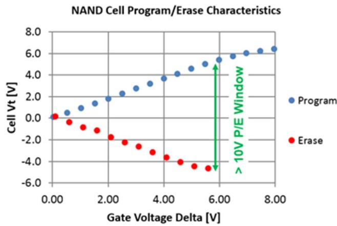
Fig. 2. NAND Cell Program / Erase characteristics
