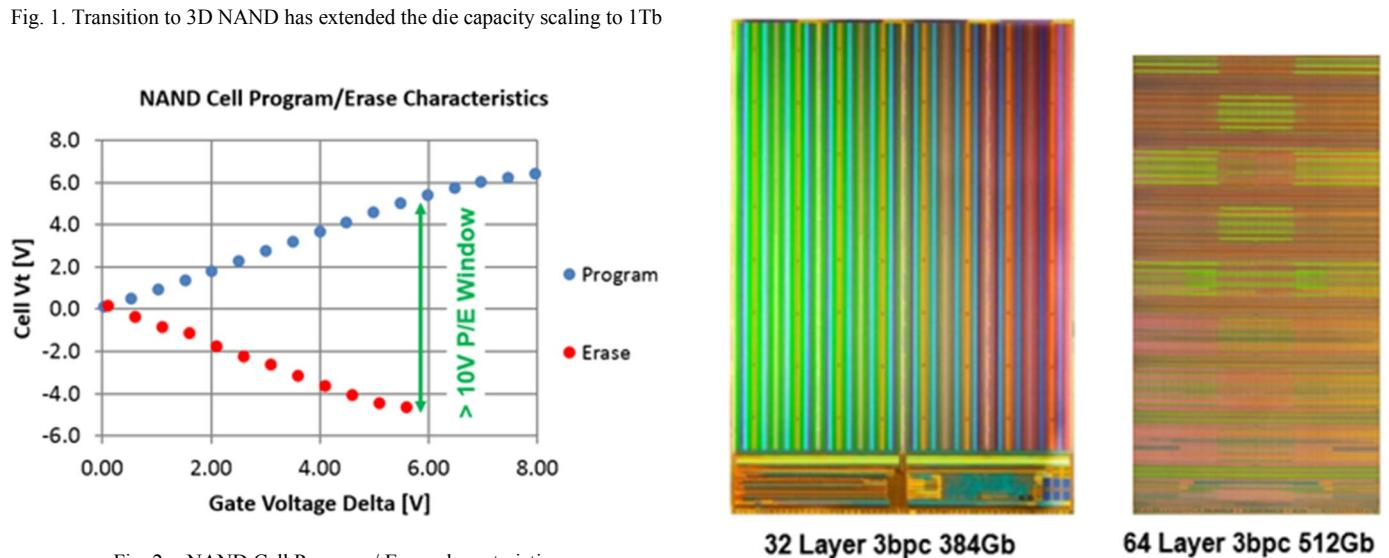
Fig. 5. Layout improvement between 1<sup>st</sup> and 2<sup>nd</sup> Gen to fit majority of circuits under the NAND Array.
