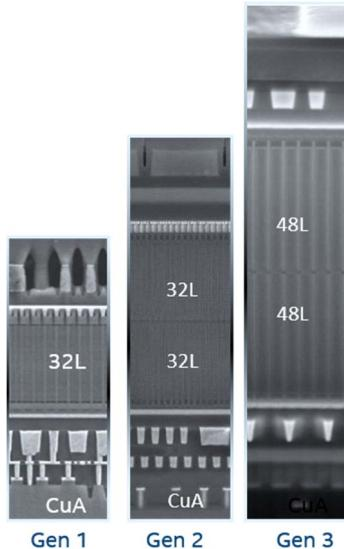
Fig. 3. SEM cross sections of FG 3D NAND with 32, 64, and 96 active layers and CMOS Under Array
